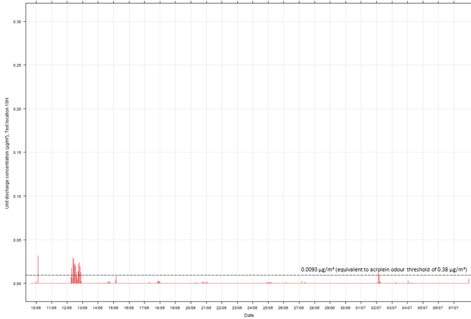
Test location 18H; Hourly average unit discharge concentrations ( \mu\text{g}/\text{m}^3 )
