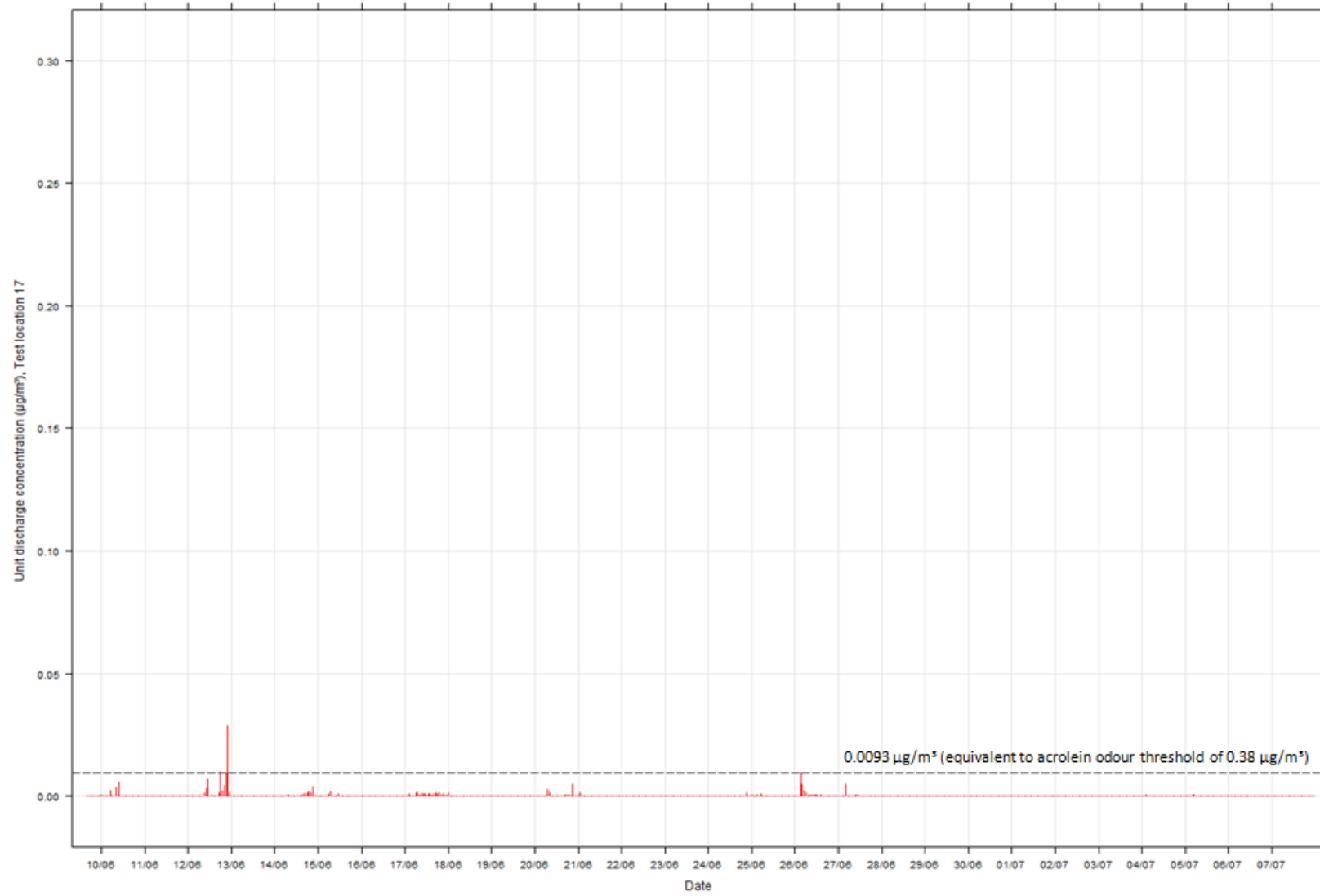
Test location 17; Hourly average unit discharge concentrations ( \mu\text{g}/\text{m}^3 )
