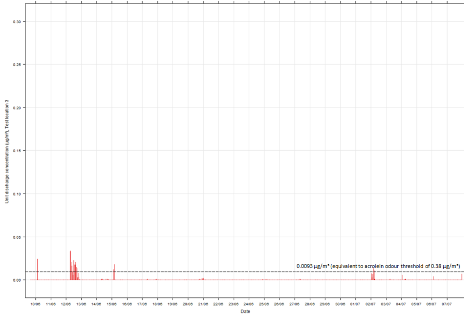
Test location 3; Hourly average unit discharge concentrations ( \mu\text{g}/\text{m}^3 )
