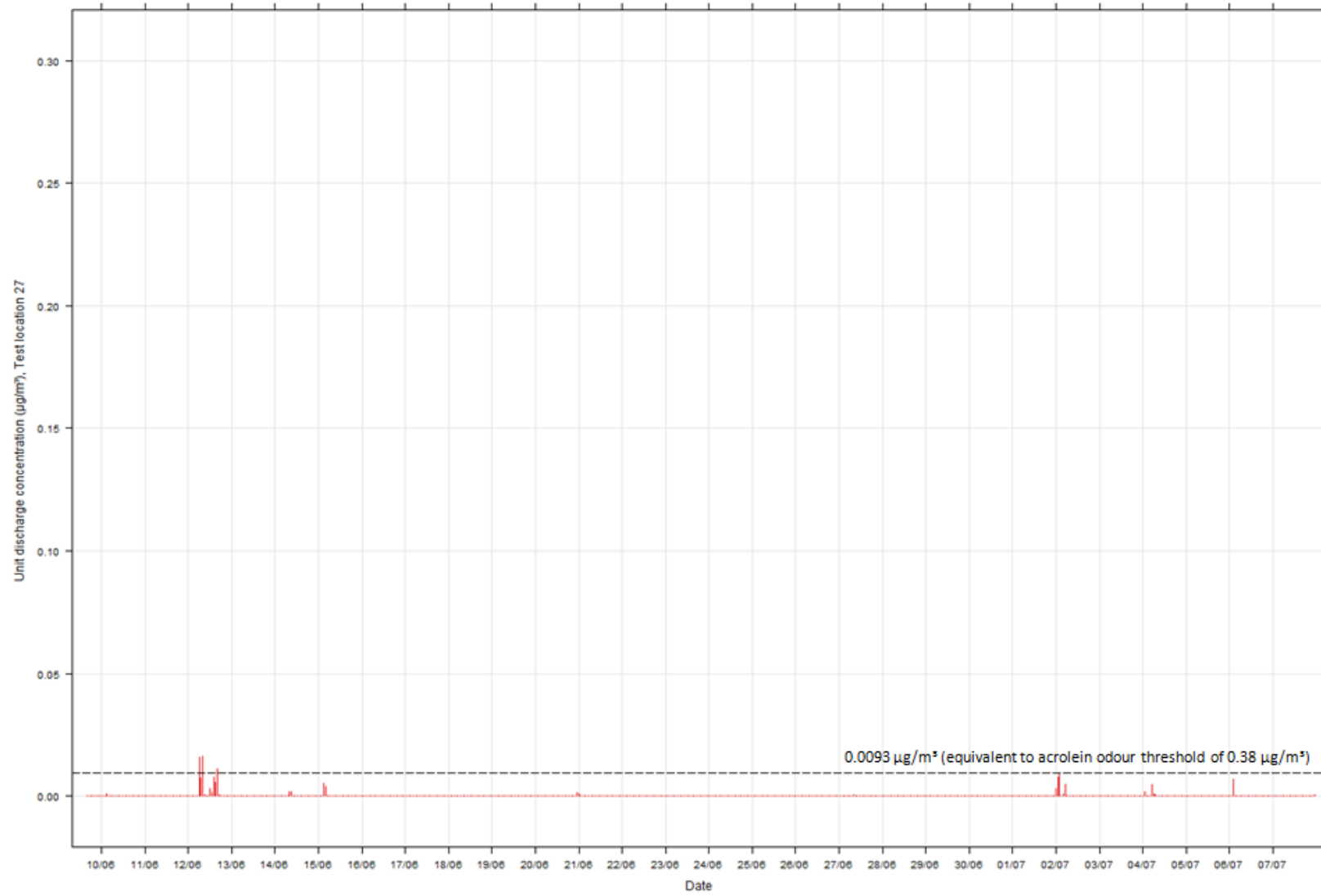
Test location 27; Hourly average unit discharge concentrations ( \mu\text{g}/\text{m}^3 )
