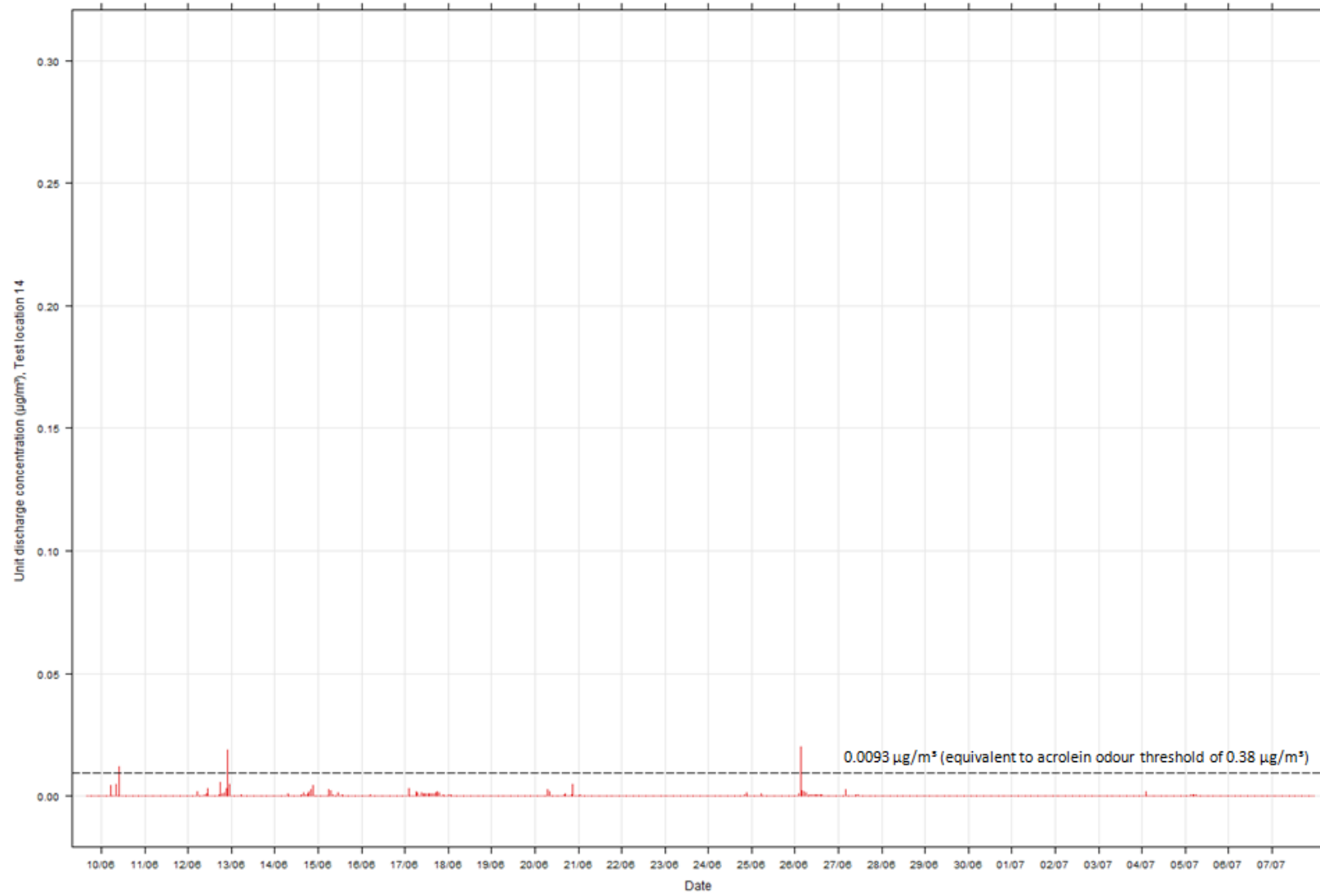
Test location 14; Hourly average unit discharge concentrations ( \mu\text{g}/\text{m}^3 )
